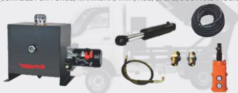
Hydraulic Power Pack 12V / 24V / 48V with solenoid release valve, check valve, relief valve & flow control valve, pump flow 1 cc / 2 cc with maximum pressure of 170 bar with oil reservoir of 15 ltrs. with hydraulic cylinder, battery & electric cable, adaptor, hose pipe & pendant switch.
